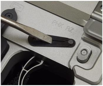
Place flat blade screwdriver in slot
