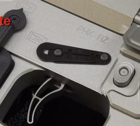
Line up flat end of pins with "D" shaped holes on back plate Then place master link over plate
